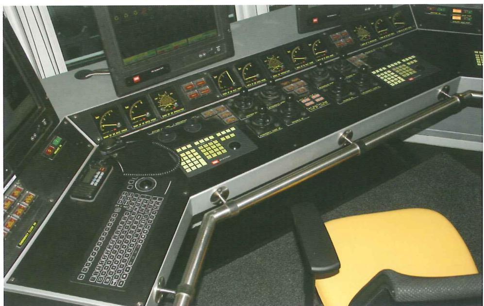
ring configuration (this configuration enables two possible paths between connections). All computers (two servers, master and backup, plus eight operational posts distributed around the ship) are connected to this network
